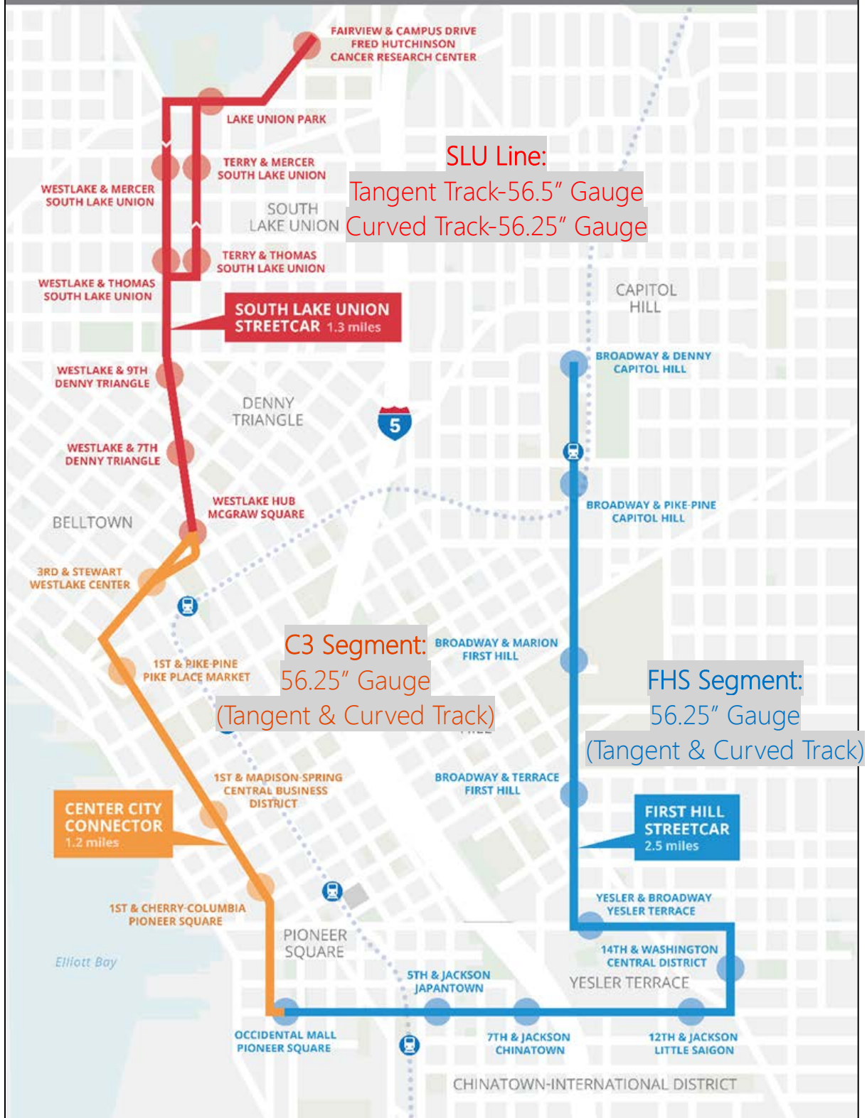
Figure 2: Existing and proposed track gauge on Seattle Streetcar segments.
