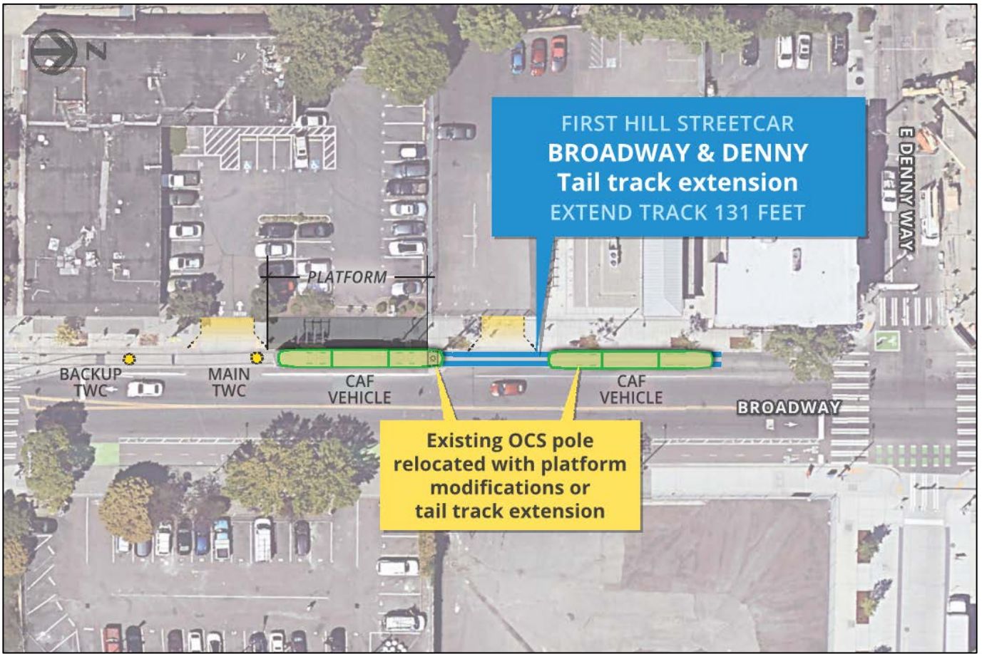
Figure 6: Conceptual design of modifications to the Broadway and Denny tail track.
